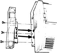
9) Install the Quick Reference Guide holder on the handset holder Push it until it snaps into the place.
